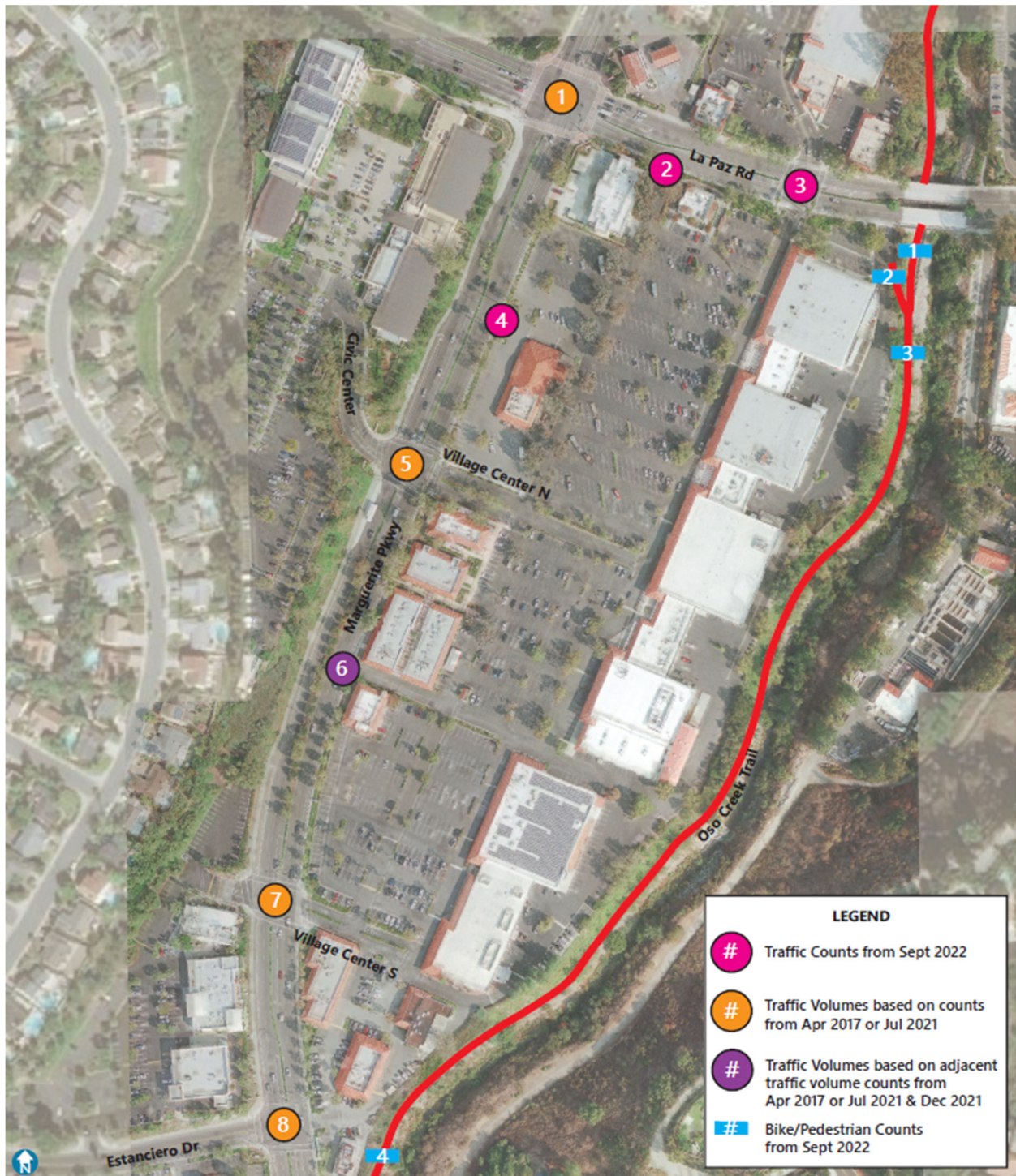
FIGURE 2.3 – EXISTING TRAFFIC COUNT LOCATIONS
